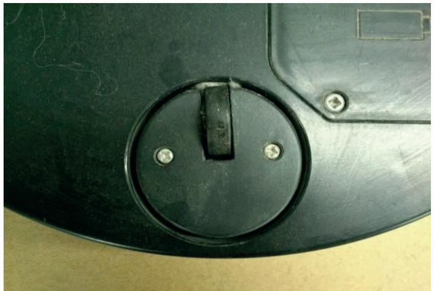
2: Take out the hair and dust. During this process, make sure do not break PCB cable
