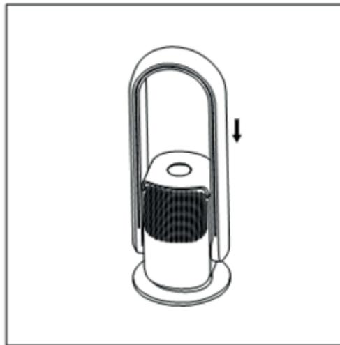
4. Reposition the filter cover: the click of the magnets placed on the cover will indicate the correct positioning.
